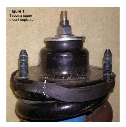
**D.** Using an appropriate spring compressor, compress the spring until it can be rotated freely by hand. Then, disassemble the shock and spring unit.
