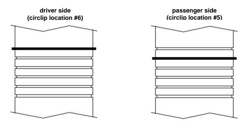
Another example: to achieve the highest lift setting of 1.75" on a **4x2 V6 Double Cab 5' bed**, the circlips should be installed as follows:
