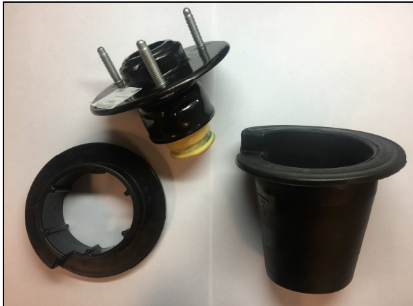
Fig 1: 2007-2013 OE GM 1500/Avalanche and 2007-2014 Tahoe Top Mount Components
