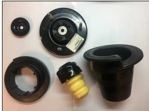
Fig 2: 2014+ OE GM 1500 and 2015+ Tahoe Top Mount Components
