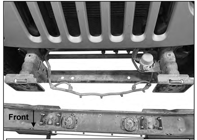
(Fig 3) Remove plastic cover from top of frame
