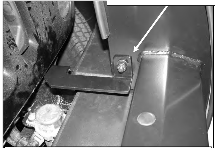
(Fig 16) All Driver/left side Top Bracket installation
