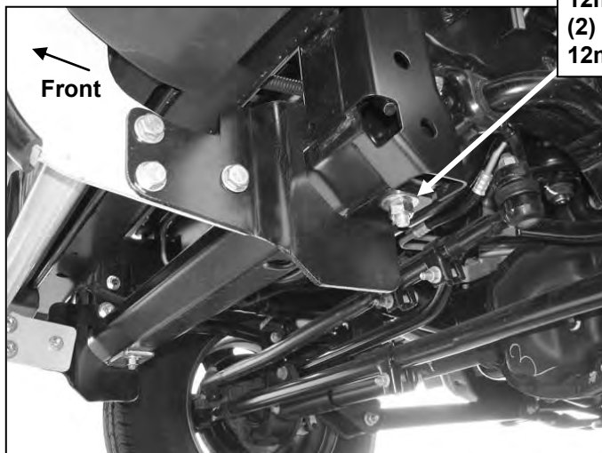
(Fig 15) All Driver/left side Frame Bracket installation
