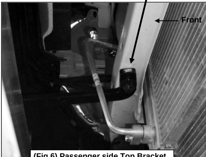
(Fig 6) Passenger side Top Bracket installation pictured from below
