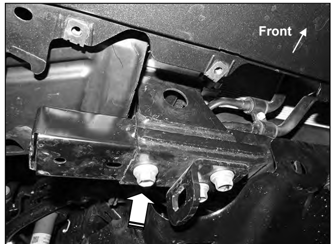
(Fig 2) Remove factory hex bolt (arrow)
