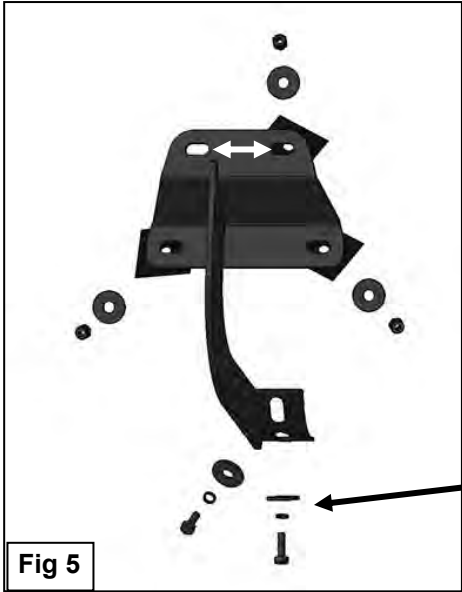
(Fig 3) Thread Plastic Washers onto all mounting studs. Driver side front pictured
