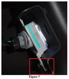
E. Install factory harness on Fab Fours bumper and insert light attached to harness into light cover and secure. Use zip-ties to secure excess wiring. Holes for securing zip-ties are located at (Ref. Figure 11)
