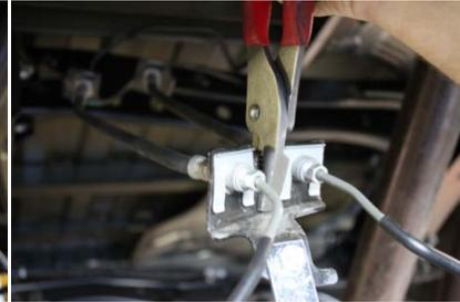
4. Release the ABS line from the bracket on the axle so that the line will be loose at full droop. (4)
