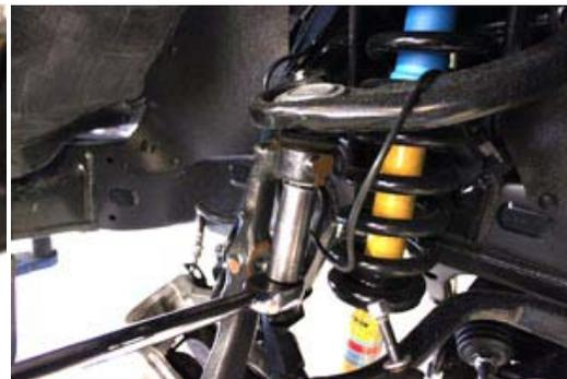
10. Remove bolts from lower ball joint / steering stop plate, then break upper ball joint loose by hitting the side of the spindle, do not hit the thread, remove stock spindle.
