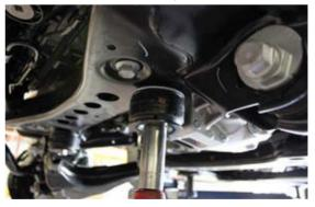
SKID PLAT SPACER INSTALLED
