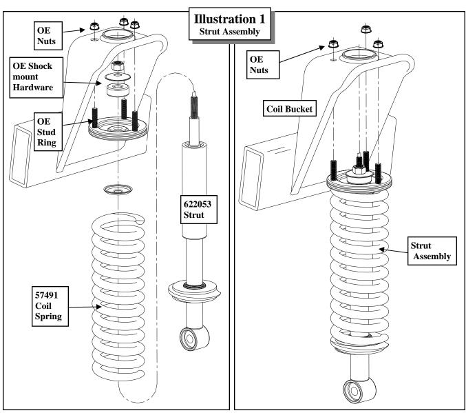
25. Recheck all hardware for proper installation and torque at this time.
