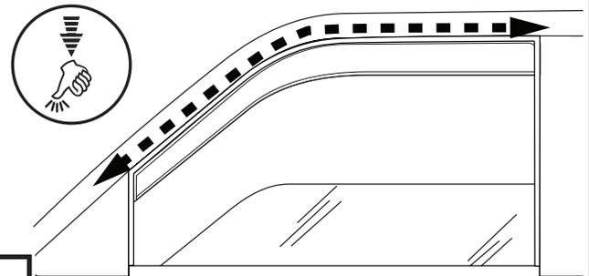
Continue to apply pressure to ensure that the visor remains properly seated inside the window channel as window is slowly closed. Leave window up for 72 hours to secure visor to window channel.
