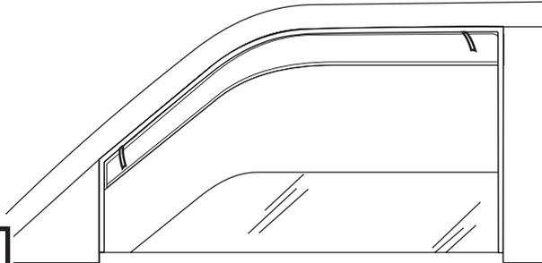
Press the exposed area of tape against the surface and verify position.
