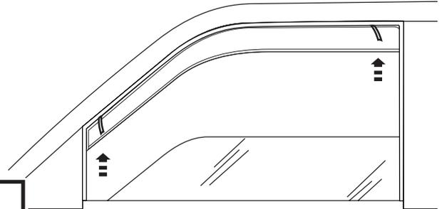
With the visor in its final position, remove the remainder of the tape liner by pulling on free ends.
