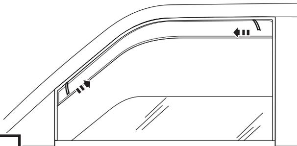
Apply pressure along the inside of window channel and flange edges to secure in place.
