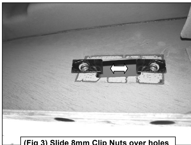
(Fig 3) Slide 8mm Clip Nuts over holes
