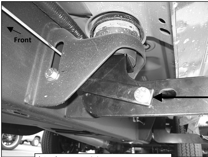
(Fig 6) 1500 Model Center Support Bracket Installation Pictured
