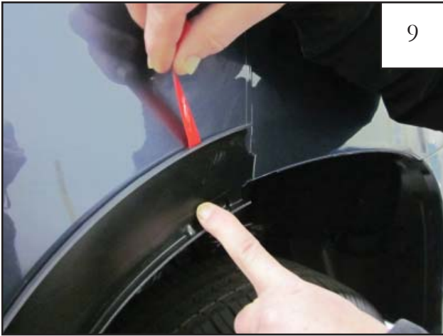
Pull remaining red tape liner and press the Inner Door Piece firmly to ensure proper tape adhesion.
