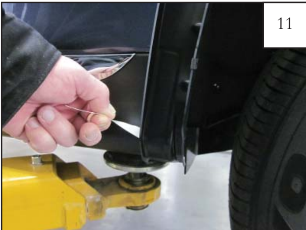
Pull remaining white tape liner and press the Inner Door Piece firmly to ensure proper tape adhesion.
