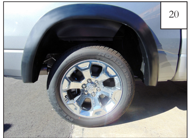
Completed rear flare installation.
