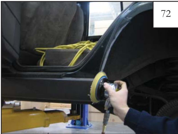
72 Open door. Sand the chipped paint along bent edge of the wheel well.
