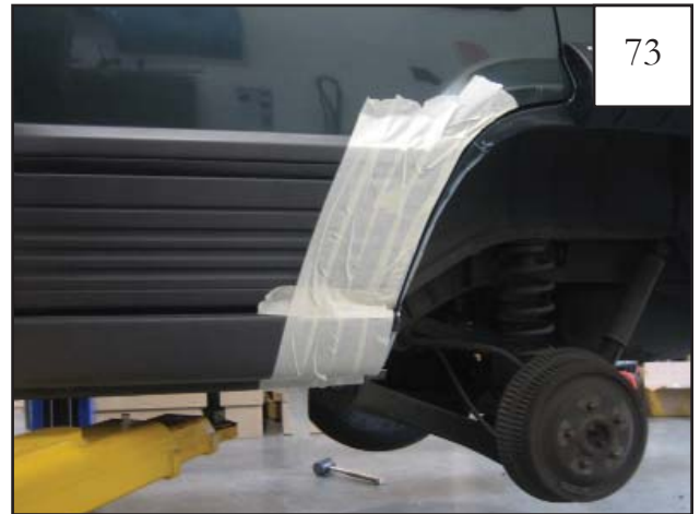
73 With door open, run masking tape along door edge. Close the door and tape over the side cladding and rocker panel.
