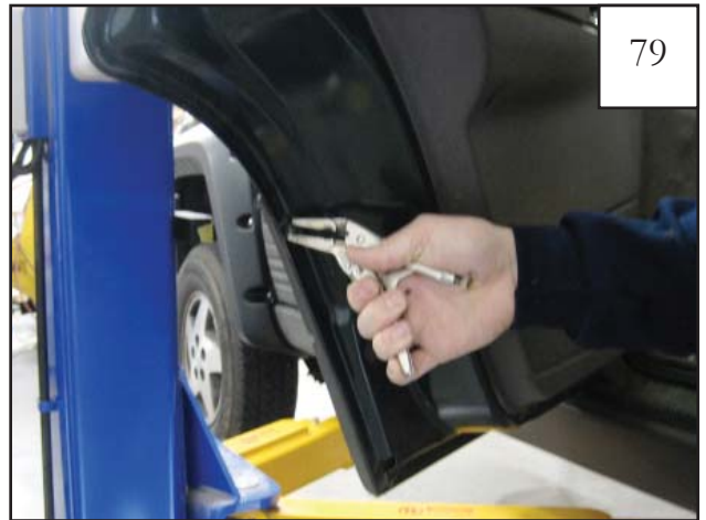
Remove nut from screw on inside edge of door with pliers or vice grips.
