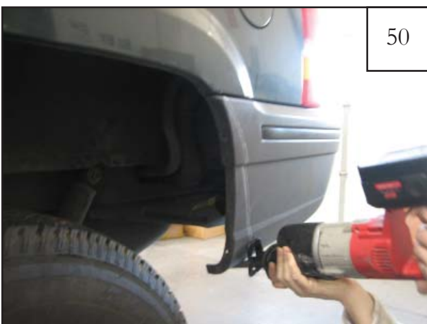
Using the reciprocating saw, cut bumper along offset line. Clean edge with a utility knife.
