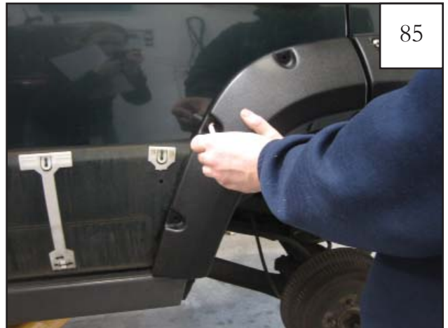
Hold door piece in place on door aligning it with rear main flare and mark hole locations onto door through holes drilled in pockets of flare.
