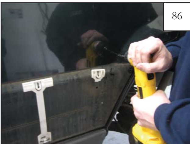
Drill holes at marks in door with 3/16" drill bit.
