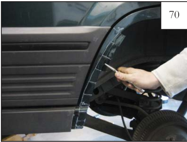
70 Bend wheel well lip out with pliers to roughly match outer face of fender.
