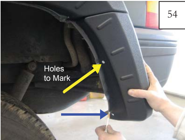
Hold the flare and bumper piece to the vehicle so that the bumper piece barely overlaps the cut bumper. Mark the locations of the lowest hole & second highest hole on the bumper. Hole locations are white in picture for visibility. NOTE: See Step 46 about gapping between bumper and bumper piece.
