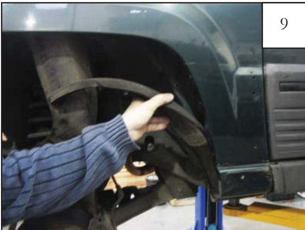
Remove and save sound dampening foam from inner wheel well. NOTE: If debris is present in inner wheel well, remove before continuing installation.
