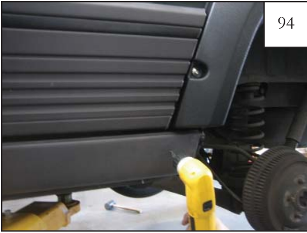
Drill marked hole through rocker panel plastic and into sheet metal underneath with 3/16" drill bit.
