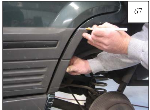
Hold factory side cladding to "dog leg" area of wheel well and trace a line at the top of the cladding on the vehicle.
