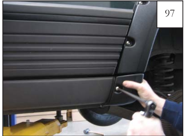
Place rocker panel flare on rocker panel aligning it with bottom of door piece. Using the provided torx bit driver, snug screw to vehicle. Torque to 24 in•lb (2 ft•lb).
