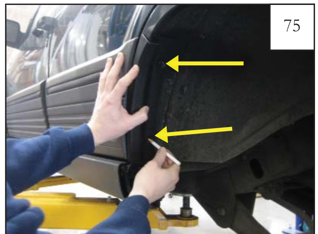
75 Hold cover piece over "dog leg" and mark inner wheel well through holes in part. If cover piece fits poorly more hammering is needed. Part is marked on the inside. Driver's side: LR5 for cover piece.
