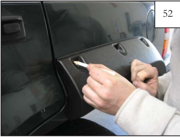
Hold flare in place on vehicle, mark hole locations onto fender through holes drilled in pockets of flare.
