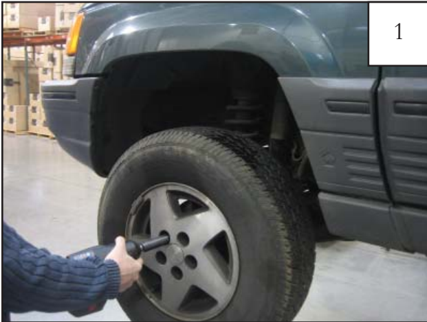
Remove tire using an impact wrench.
