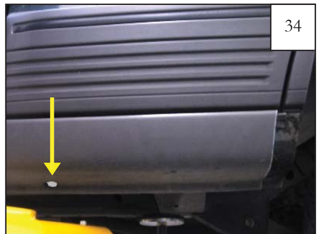
Slide rocker panel forward (approximately 10 mm) until the christmas tree faster in the slot on the underside stops movement. Fastener is white in picture for visibility.
