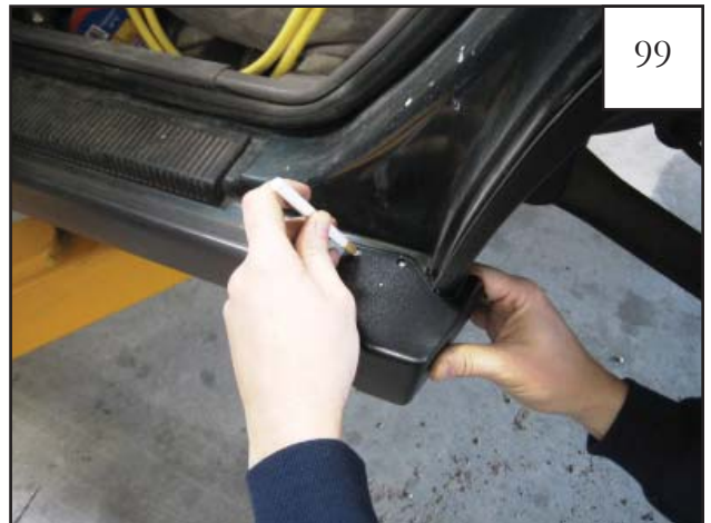
With door open and rocker panel piece held in position, mark hole locations on door sill through holes in rocker panel piece.
