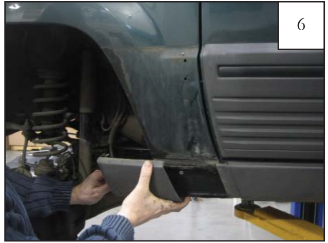
Remove lower factory side cladding piece from front fender.
