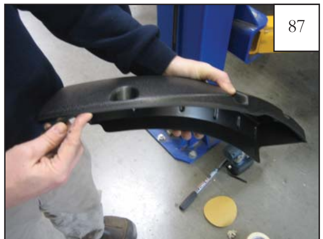
For edge trim (GP1-0005) application on rear door piece, follow steps as listed at the beginning of this instruction set. Apply edge trim only to the outer edge of the door piece.
