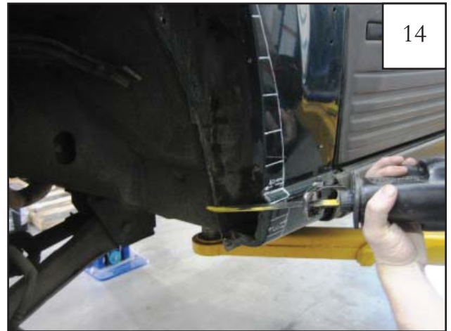
Starting at the style line, cut along horizontal marks from wheel well to vertical line with reciprocating saw.
