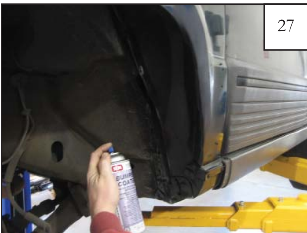
Using spray paint, repaint the sanded edge of the wheel well flange. NOTE: Be sure to cover the rest of the vehicle so paint does not get on other accessories such as side cladding.
