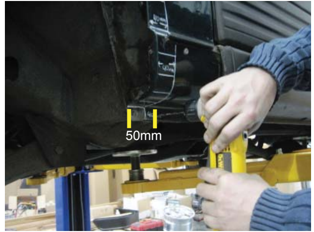
Approximately 50mm back from lip, predrill a hole through the pinch weld using a 3/16" drill bit.
