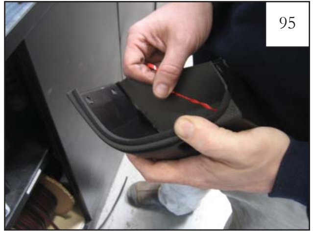
For edge trim application on rocker panel piece, follow steps as listed at the beginning of this instruction set. Apply edge trim only to the door piece along edge that will be closest to the front of the vehicle. Part is marked on the inside. Driver's side: LR4 for rocker panel piece.
