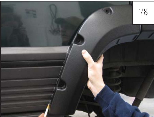
Close rear door. Hold door piece in place on door aligning it with rear main flare and trace outer edge of flare onto body side molding. Part is marked on the inside. Driver's side: LR3 for door piece.
