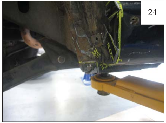
Cut along horizontal lines in pinch weld using reciprocating saw.
