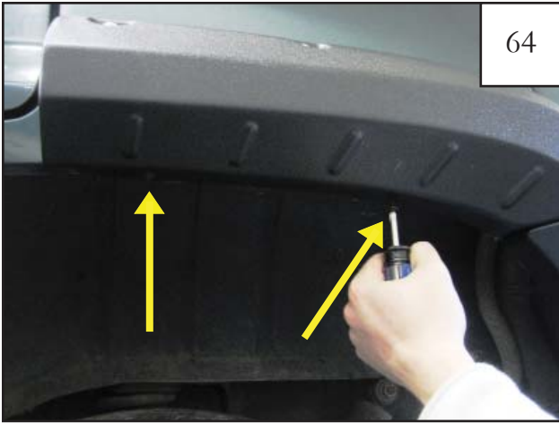
Secure flare to fender with the #8 pan head screws (SW1-0056) through holes in flare and into predrilled holes. A drill with a #2 Phillips driver works well.
