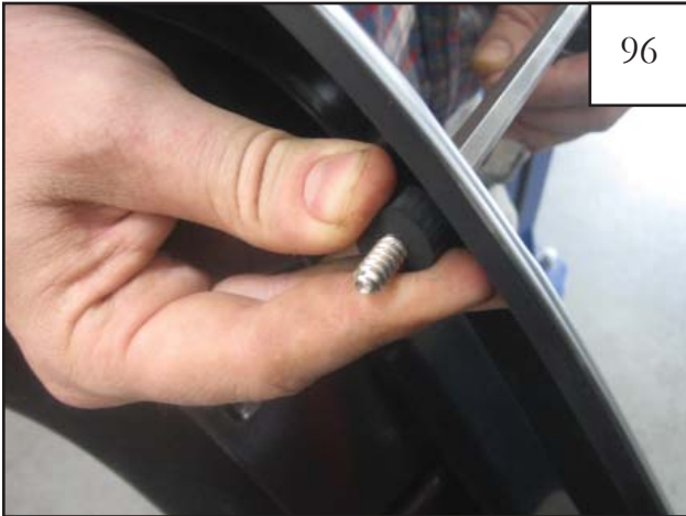
Put screw (SW1-0045) through hole in pocket of rocker panel piece and secure with rubber grommet (SP1-0009) using supplied #45 Torx bit. Drive screw into grommet until tight.
