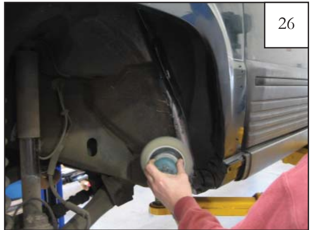
Sand bent edge of pinch weld.
