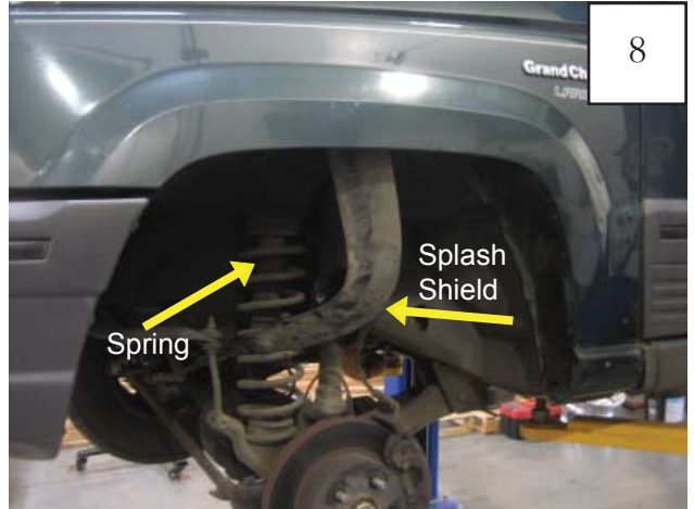
Pull the splash shield away from rear area of the fender and tuck it into the spring.
