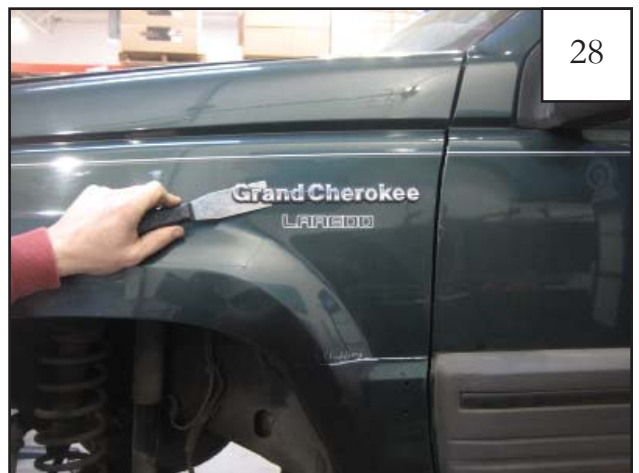
Using a putty knife, remove any decals. Buff residual adhesive off with adhesive remover disk.
