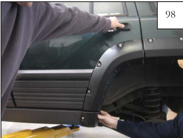
Align rocker panel piece to bottom of door piece by hand and hold in position. Have a partner open the door.
