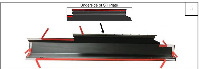
Peel back roughly 3" of red tape liner from the pieces of tape on the back side of the front part. Make sure red tape liner will be accessible when part is attached to truck.
