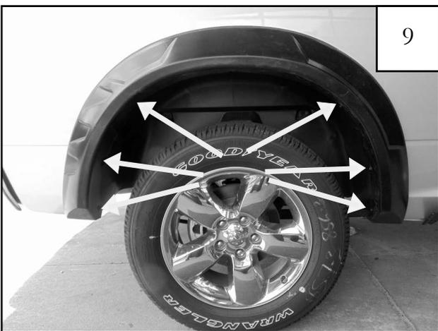
Hold flare in place while you start previously removed factory screws using an 8mm socket. *Do not tighten.*
