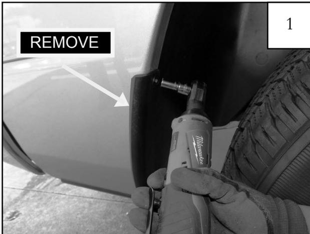
If you encounter a fit problem, remove inner piece at bottom rear and front of wheel well.
