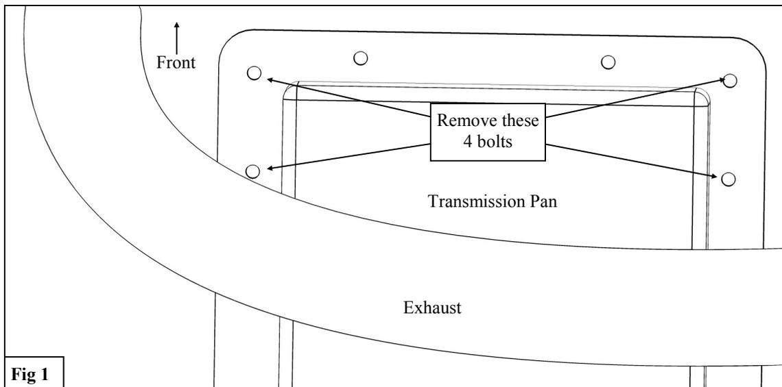
3. Loosely install Brackets A & B (3,4) using the supplied M6 Hardware in the driver side bolt locations shown in **Figure 1**. See **Figure 2**.
