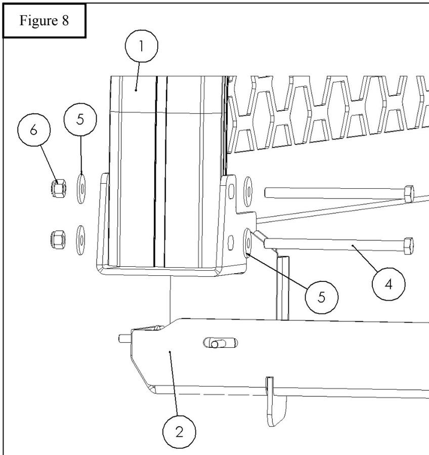
Note: When tightening M8 hardware that was used to install hoop and screen assembly on step 8, push the top of the HLR rack towards the cab of the truck to maintain straight while tightening.
