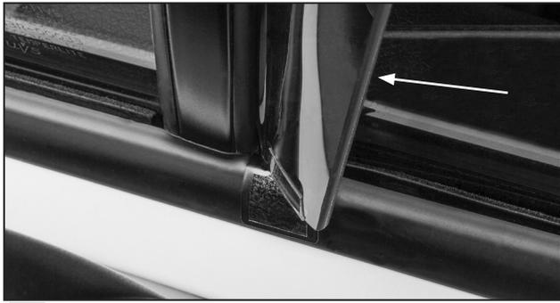
**5** With the deflector now resting on the weather strip clip, slide forward into the channel. Ensure edge rests on top of the weatherstrip clip.
