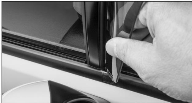
**4** Lower the front of the deflector onto the weather strip clip as shown.
