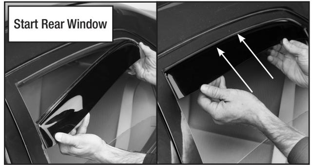
**10** Be sure to remove adhesive backing before installation (if supplied). Slide upward into place, then gently pull outward to set the deflector.
