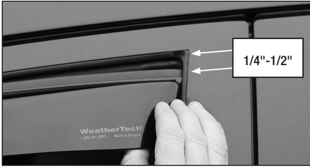
**7** Insert the rear edge leaving a gap at the top.
