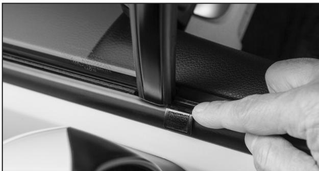
**3** Place the weather strip clip onto the window gasket material: position as far forward as possible.
