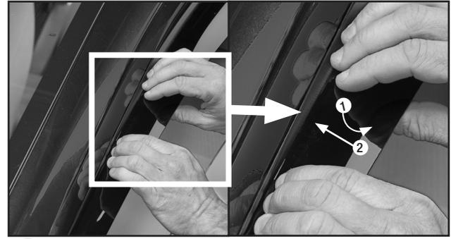
**8** Pull down and tuck in working from front to back.
