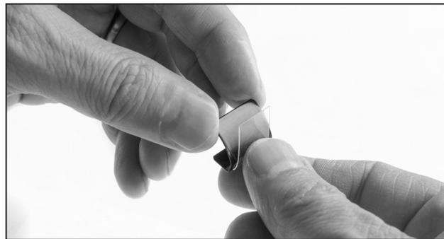
**2** Place one strip of the provided clear tape centered onto the top of the weather strip clip.
