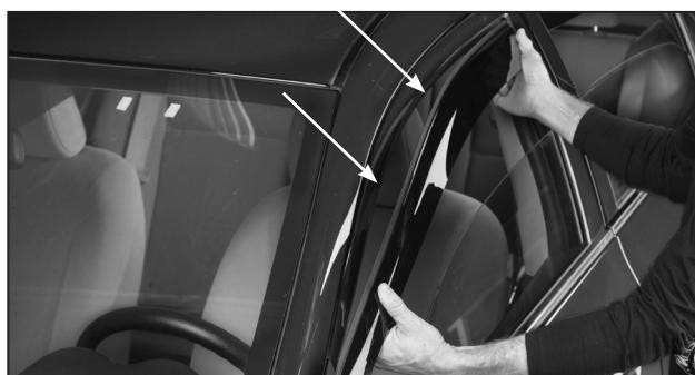
**2** Slide forward, into window channel. Ensure edge
