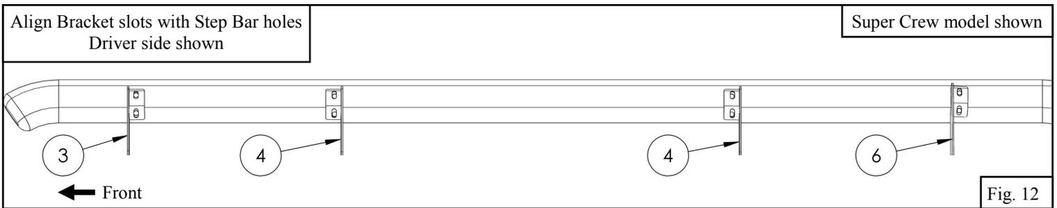
14. Align and adjust the step bar and brackets as necessary then tighten and torque all fasteners as follows: M8 to 20 ft-lbs, M10 30 ft-lbs.
