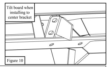
(NOTE: Reference for bracket locations and orientations can be found below in Figures 13-16 and on pg. 5)
