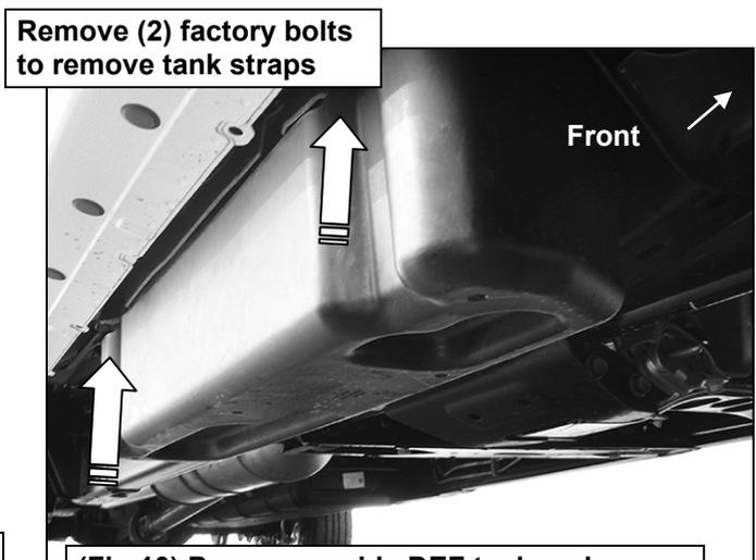
**(Fig 10) Passenger side DEF tank and cover**
