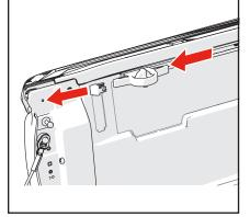
Install the cab slide block (B) into the rear (tailgate) end of the cargo rail. Position near the cab. Align the cab clamp bracket (C) with the cab clamp of the bed cover. Use the Torx screws (D) to mount the cab clamp bracket (C) to the cab slide block (B). Tighten the screws with the T-27 Torx tool. Do this for both sides of the truck bed.
