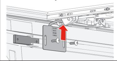
Adjust the rear (tailgate) striker bracket (I) so that it aligns squarely with the cover latch. Push down on cover when tightening the Torx screws (E) so that the rear (tailgate) striker bracket (I) pulls the cover down tightly to the truck bed cap. Do this for both sides of the truck bed.
