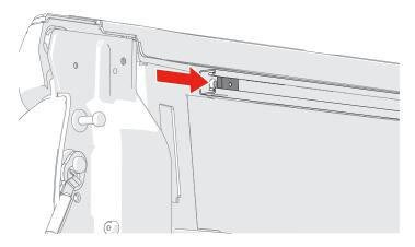
Adjust the rear (tailgate) striker bracket (G) so that it aligns squarely with the cover latch. Push down on cover when tightening the bolt and screws (E) so that the rear (tailgate) striker bracket (G) pulls the cover down tightly to the truck bed cap. Do this for both sides of the truck bed.
