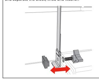
Reassemble the tether by threading the knob through the washer and into the slide block. Install the tether on both sides of the bed.
