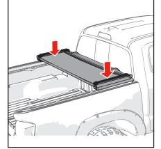
Unfold the bed cover (A) fully and adjust its position over the truck bed for the proper front (cab) and rear (tailgate) alignment. When positioned front and back, the tailgate seal should contact the tailgate with the first two fins.
