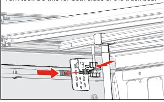
Hook the cab clamp under the cab clamp bracket (C) and tighten the T-handle until it contacts the bracket (C), then tighten two more turns. Do this for both sides of the truck bed.
