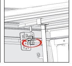
The tether comes assembled on the cab bow of the bed cover. Unscrew the knob from the slide block and separate the block, knob and washer.
