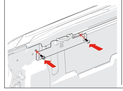
Install the Tacoma short slide block (F) for the rear (tailgate) striker bracket (G) into the end of the cargo rail.
