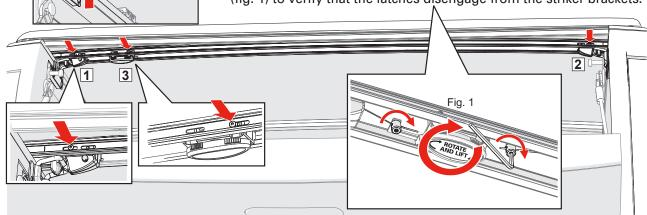
Double-check that the cover is secure and tight to the truck bed by gently lifting the corners to ensure the mechanisms are engaged.
