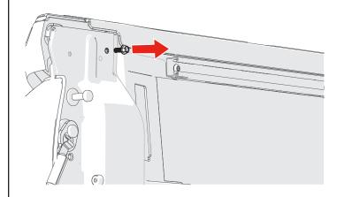
Install the Tacoma rear (tailgate) striker bracket (G) using the factory bolt reinstalled into the same hole from where it was removed and the Torx screw (E) threaded into the slide block (F).
