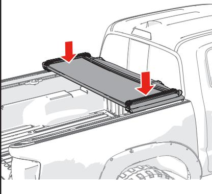
**8** Unfold the bed cover (A) fully and adjust position over the truck bed for proper front (cab) and rear (tailgate) alignment. When positioned front and back, the tailgate seal should contact the tailgate with the first two fins.
