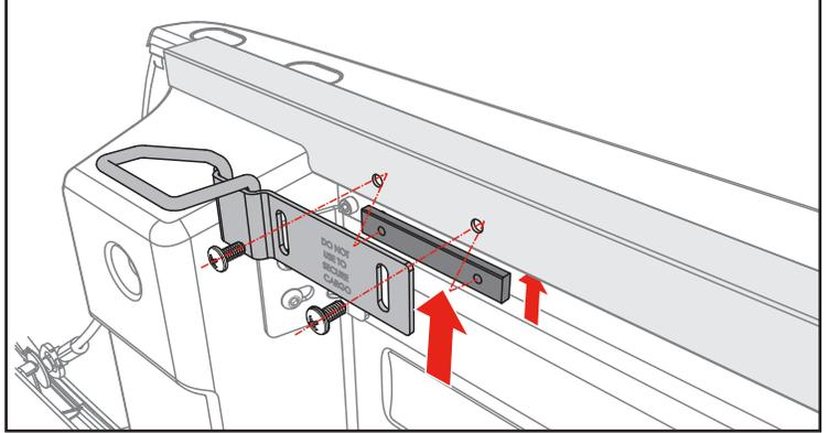
**12** Install the striker brackets (J) on both sides of the truck. Leave the screws (L) loose for later adjustments.
