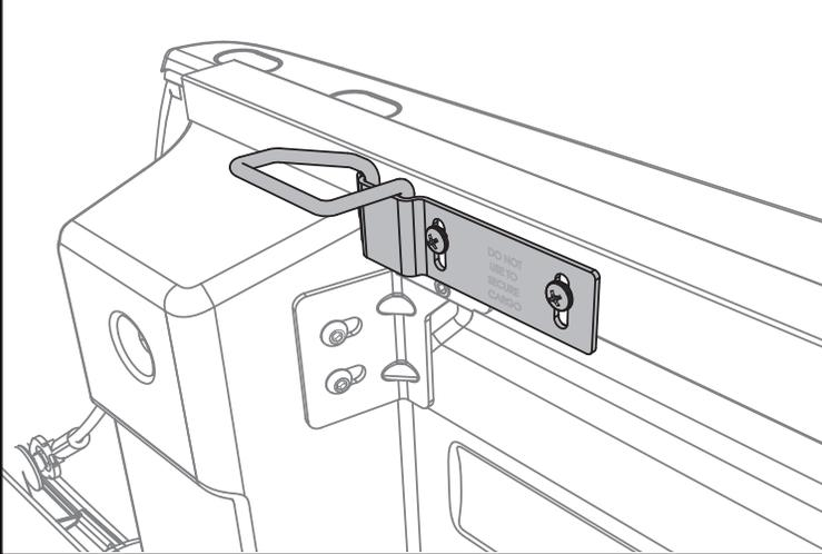
**13** Close the bed cover (A), align the latch with the striker bracket (J) and tighten the screws (L) with a Phillips screwdriver. Push down on the cover (A) while tightening.
