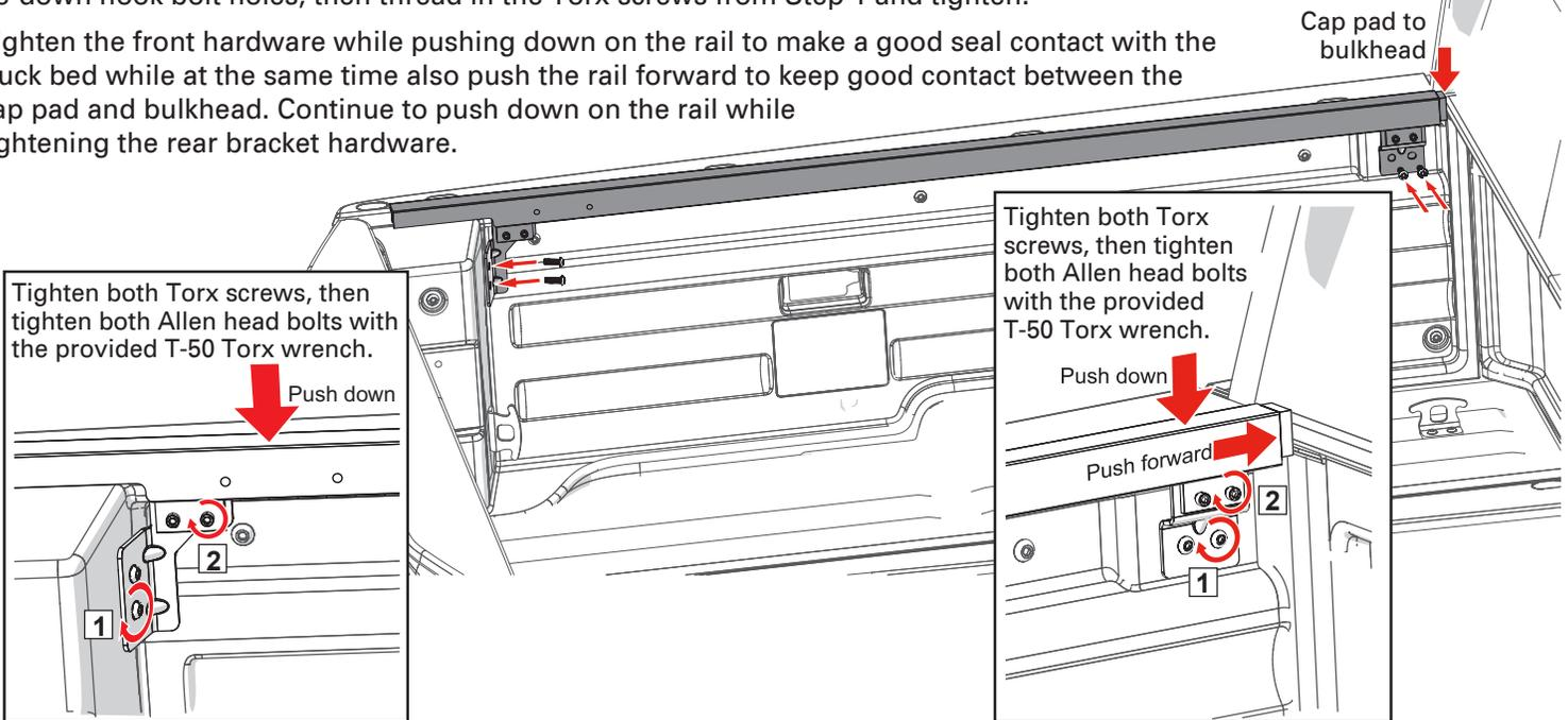
**7** Place the folded cover (A) on the cab end of the truck bed. Make sure the cover is square with the truck bed and the bulkhead seal sits on the truck bed bulkhead.
