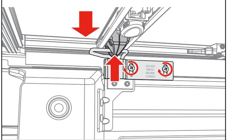
**14** Adjustments and tightening of the latch assembly is required.
