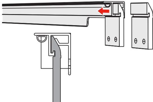
**4** Slide one rail bracket (D) towards the cab, leaving the other at the tailgate of each rail (B & C).
