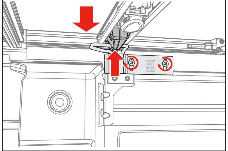
**17** The tethers come installed looped over the bed cover bow with a snap hook at the other end. Hook the tether onto the truck bed tie-down. Install the tethers on both sides of the cover.
