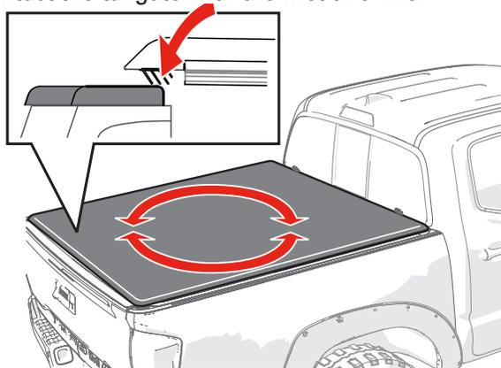
**9** Carefully refold the bed cover (A) without shifting its position on the truck bed.
