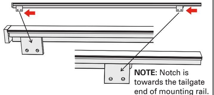
**5** With the rail brackets (D) slid into the rails (B & C), assemble the full brackets as shown. Loosely tighten the screws (G) with provided 3/16" hex wrench.
