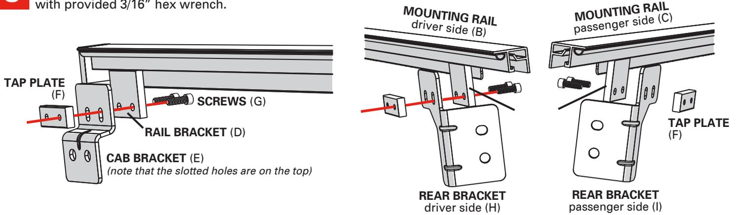
**6** Place the rails (B & C) on the truck once the brackets are mounted to the rails. Position the rails (B & C) so the front cap pad firmly contacts the bulkhead. Align the brackets so they line up with the factory tie-down hook bolt holes, then thread in the Torx screws from Step 1 and tighten.
