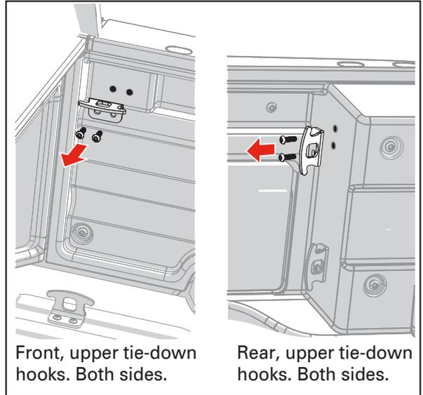
**2** Align the parts for assembly as shown.
