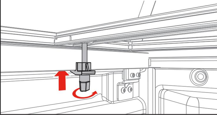
**11** At the tailgate attach the striker brackets (J) to the mounting rails (B & C) by threading the screws (L) through the striker bracket (J), through the rail (B & C) and into the slide block (K).
