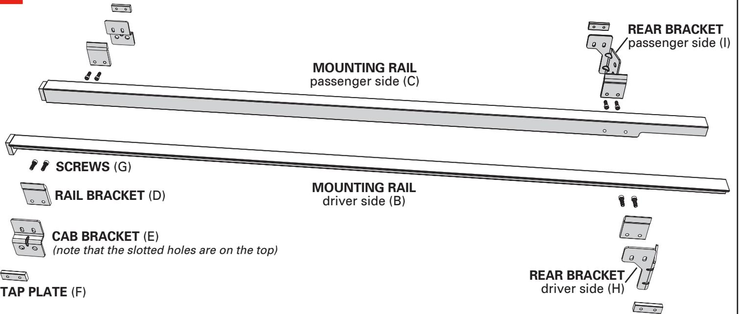
**3** Slide two of the rail brackets (D) into each rail (B & C). Align with the rail interior profile as shown.
