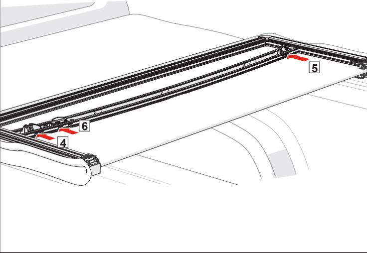
**16** To make the final adjustment, loosen the striker bracket screws. Then move the bracket down by firmly pulling the cover to the truck rail and tailgate. Make sure that both sides match, then retighten the screws.
