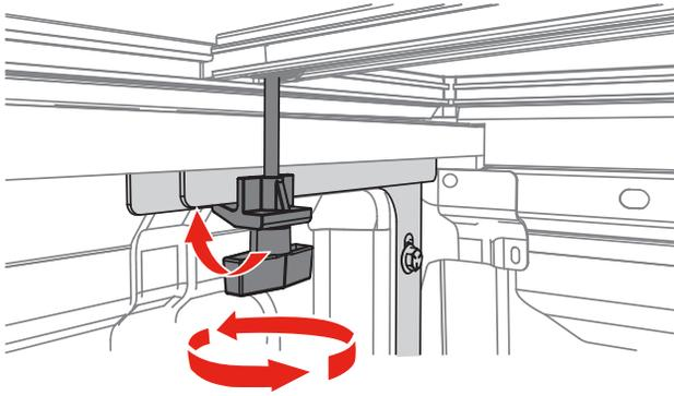
Hook the cab clamp under the installed cab rail brackets (G). Tighten the knob until the jaw makes contact, then turn an additional two turns. Repeat on the opposite side of the truck bed.
