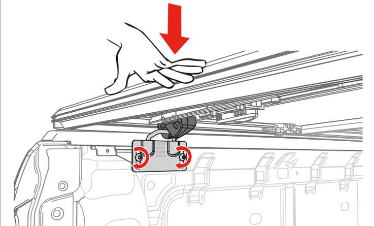
**13** The tethers come installed looped over the bed cover bow with a clamp at the other end. Install the clamp end by sliding the clamp onto the truck rail. Make sure the clamp is positioned as far up onto the rail as possible. Firmly hand tighten the knobs. Install the tethers on both sides of the cover.
