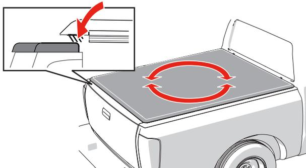
**3** Carefully refold the bed cover (A) without shifting its position on the truck bed.
