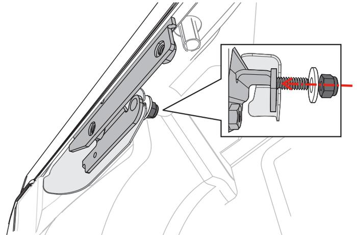
**7** Attach the striker bracket (C) to the latch bracket (D) using the Torx head screws (B). Leave them loose for later adjustments.
