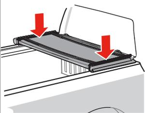
**2** Unfold the bed cover (A) fully and adjust position over the truck bed for proper front (cab) and rear (tailgate) alignment. When positioned front and back, the tailgate seal should contact the tailgate with the first two fins.
