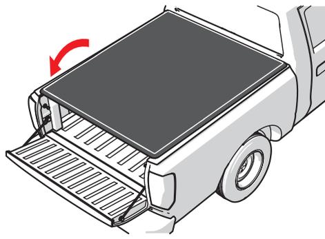
**9** Align the latch with the tailgate striker bracket (C). Push down on the cover while tightening the Torx screws (B) with the supplied T-27 wrench.
