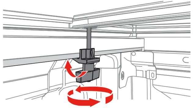
Hook the cab clamp under the truck bed rail metal flange. Tighten the knob until the jaw makes contact, then turn an additional two turns. Repeat on the opposite side of the truck bed.
