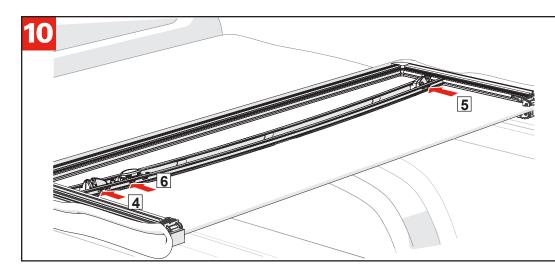
Fold the panel open and tighten the rear T-20 Torx screws in both the driver and passenger side latches and the actuator mechanism, shown below as 4, 5 & 6.
