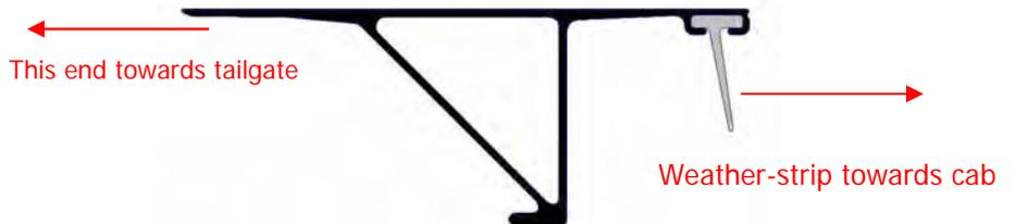
**STEP 4 Install the front cover.** The front cover is attached below the rails. Hold the cover level and push both ends in evenly to help slide it into place. When the holes are lined up, start threading the (2) **Front Cover mounting screws**. Tighten the 2 screws securely using the enclosed 1/8" Allen wrench.
