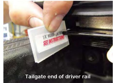
**STEP 9 Bolt rails to pickup bed rails.** Position rail spacer block and cleat inline with the hole in the rail. Start threading bolt with washer into cleat. Repeat at other 3 mount locations. Keep rail level when tightening bolts
