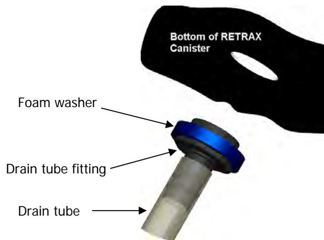
**STEP 12 (b)** Finish Installing the drain tubes. On some models there are factory drain holes in both front corners, on others there are plastic plugs that can be drilled out for the tubes. You can enlarge existing holes or drill new holes in the front wall or floor if needed. Be careful of what is behind when you drill. If using a plastic bed liner, then holes need to be drilled through the liner only. Cut the tubes to length to fit in desired locations.
