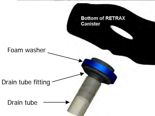
**STEP 12 (b)** Finish installing the drain tubes. On Tundra models there are (2) black factory plastic plugs in the front wall of the bed that can be drilled or cut for the tubes. If using a plastic bed liner, then holes need to be drilled through the bed liner only. Cut the tubes to length to fit in desired locations.
