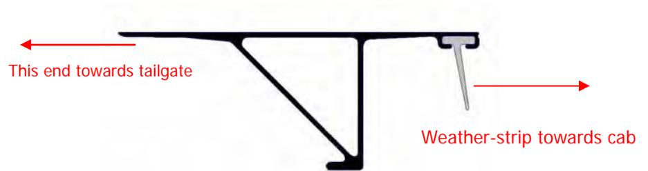
**STEP 4 Install the front cover.** The front cover is attached below the rails. Hold the cover level and push both ends in evenly to help slide it into place. When the holes are lined up, start threading the (2) **Front Cover mounting screws**. Tighten the 2 screws securely the enclosed 1/8" Allen wrench.
