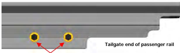
To adjust the distance between the rails, remove the clamp and turn both of the white nylon adjustment screws using a 1/4" Allen wrench.
