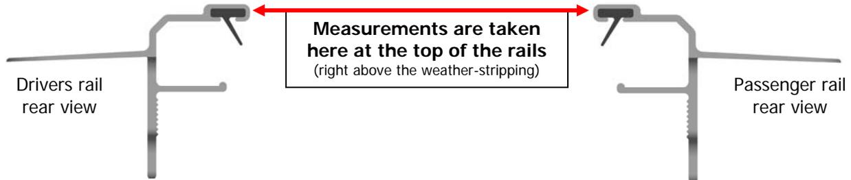
**STEP 9 a.** Measure and record the distance between the rails at **A** - next to front cover screws. This is your base measurement.
