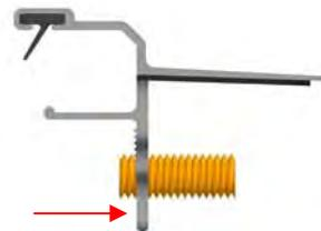
\*If the rails are too far apart, turn the adjustment screws in. (clockwise)
