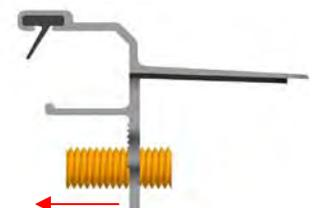
\*If the rails are too close together, turn the adjustment screws out.
