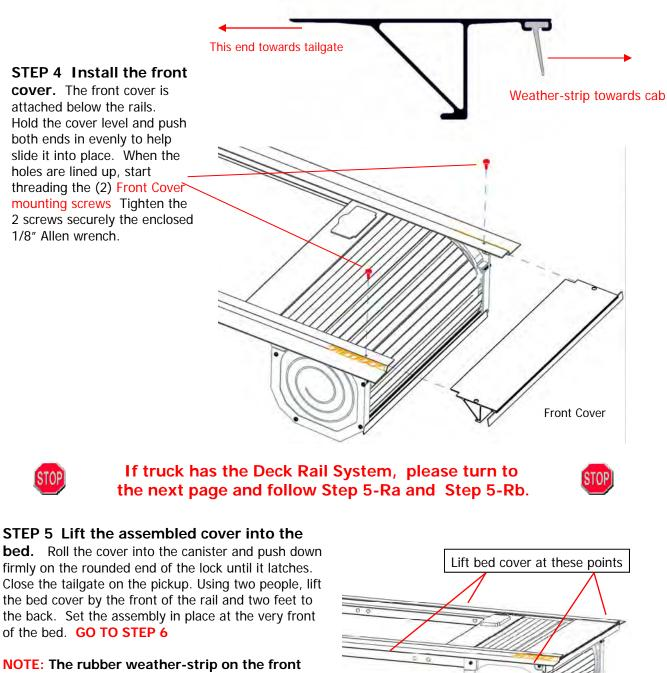
cover should lie on top of the pickup's front rail pointed towards the cab.
