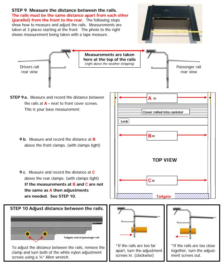
One complete turn of the rail adjustment screw equals about 1/16" of adjustment. Adjust the adjustment screws evenly between the driver's and passenger side at each set of clamps.
