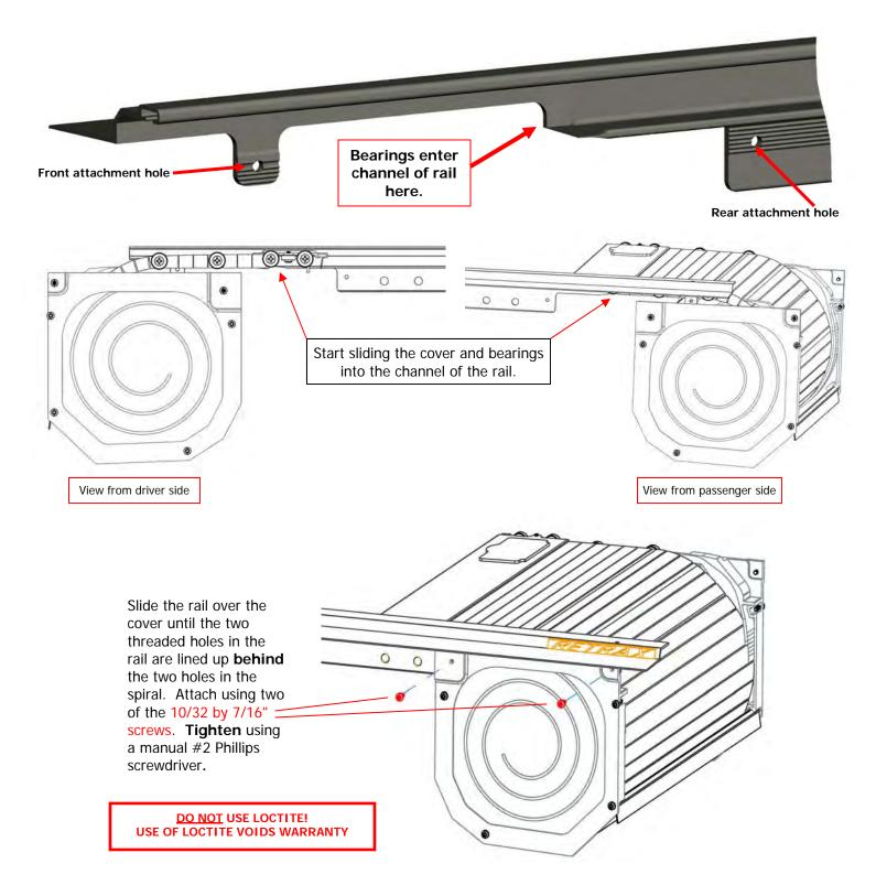
STEP 3 Install the driver rail. Lift up the lock cover and open lock by pressing release button. Pull the cover out of the canister 6"-8" (See PowertraxONE Installation Supplement on how to move electric cover). Caution: DO NOT allow cover to roll back into canister until rail is installed. Repeat Step #2 to install the driver's rail. Be sure all rail mounting screws are tight.
