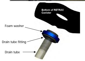
**STEP 12 (b)** Finish installing the drain tubes. On Tundra models there are (2) black factory plastic plugs in the front wall of the bed that can be drilled or cut for the tubes. If using a plastic bed liner, then holes need to be drilled through the bed liner only. Cut the tubes to length to fit in desired locations.
