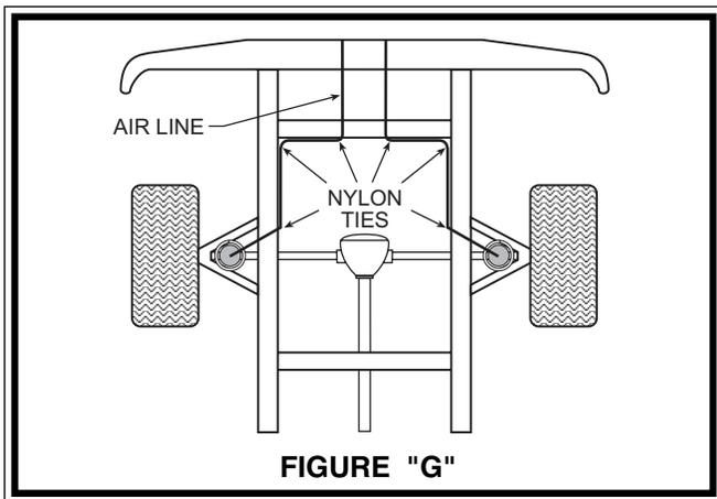
from the air spring to the desired inflation valve location.
