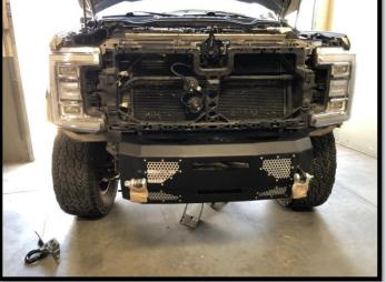
11. Once center section is on, install wings using provided washers and nuts. Best to get a friends help when installing wings to ensure proper fitment. NOTE: Install light into wings prior to installing on truck for easier light installation.
