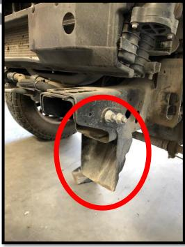
9. Install the new winch plate using factory lower scoop hardware. NOTE: If installing winch, now is the best time to do so.
