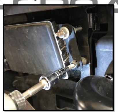
7. Unclip the fog light harness from the truck on the underside of the bumper. Remove bumper from truck. NOTE: When removing bumper, on the passenger side near the fog light is a plug for the airbag sensor, unplug to continue with bumper removal.
