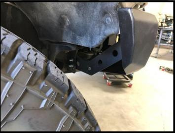
13. Once bumper is installed, if you had Adaptive Cruise Control, using relocation mount, install mounting using self-tapping screws in location shown. Using factory hardware, mount sonar in same direction as factory (plug on top towards passenger).
