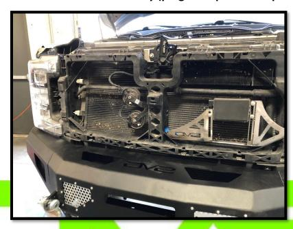
14.Reinstall grill. Depending on type of grill, place sonar in middle of largest opening.
