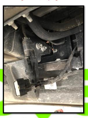
8. Remove factory tow hooks and lower frame scoops. Keep scoop hardware readily available.
