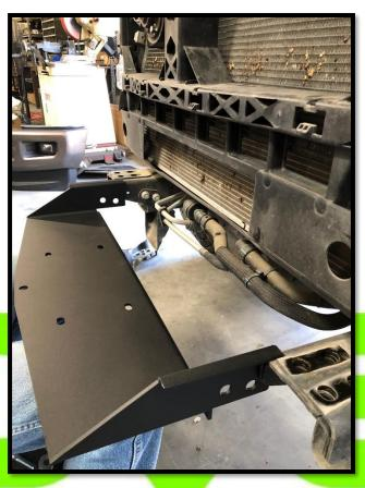
10.Install center section of bumper over winch plate using provided hardware. NOTE: If installing 10" single row light, install before mounting center section onto vehicle.
