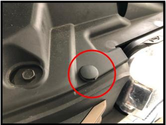
3. To remove the grill, looking from the top down on the inside you will see clips like the image below. Using a long item, push down on the clips while pulling outwards to release the clips.
