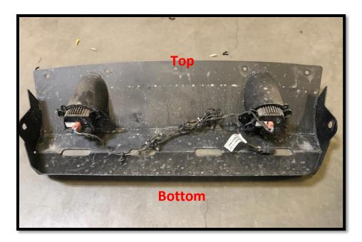
9. Install the Skid plate onto the Jeep using the provided long bolts. These bolts will go through the frame horn on each side of the Jeep. Keep bolts loose.
