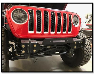
Once winch plate is secure, install the main center section of the bumper by sliding it over the top of the winch plate. The bumper should wrap over the D-Ring mounts like shown in image below.
