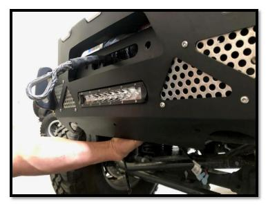
7. Install the wings (included stubby) or (full-width FBJL-02W) with the provided rock washers and hardware. The hole in the front of the stubby wing will remain open at this point.
