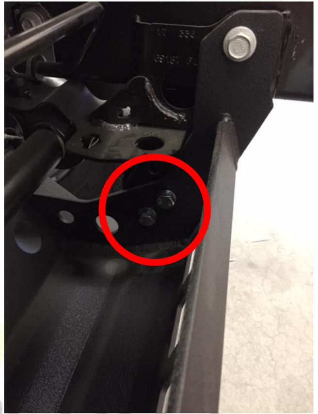
**NOTE:** Some JLs will not need the nut plates since the two holes will be threaded from the factory.
