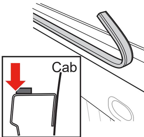
**2** Place passenger side rail (A) on the truck rail with the slotted bracket pushed all the way toward the cab and the bulkhead.
