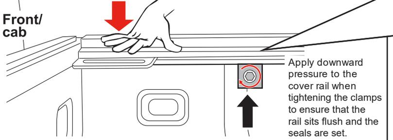
**NOTE:** When installing each clamp, make sure that the clamps are inserted as far up onto the rail as possible and that the clamp teeth fit squarely and fully engage the ribs of the cover rail.
