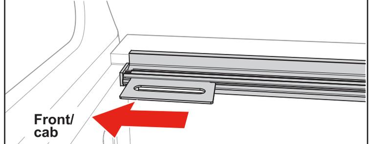
**NOTE:** Some drop-in bedliners may require trimming in the corners to fit the rail into the opening.
