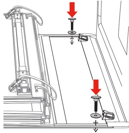
**10** Assemble the washers from underneath and **loosely** tighten the knob (M). **Do not overtighten.**
