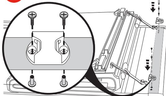
Position the buckle ends (N) so the open side faces the bed cover panel. Use a screwdriver to install the two buckles into the pre-drilled holes on the front header panel with the provided machine screws (O) and rivet nuts (P).
