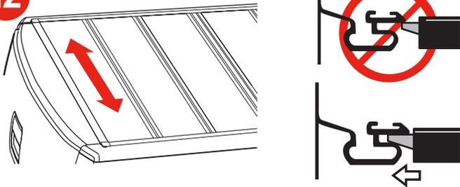
**13** The cover's aluminum frame should fit just inside the tailgate, within a 1/4" (6.4 mm) when the cover is properly positioned.
