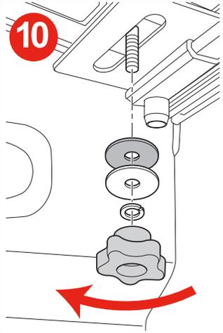
Install the washers onto the threaded shaft of the elevator bolt (I), starting with a rubber washer (J) first, then the stainless washer (K), then the lock washer (L), and finally the lock knob (M) as shown to the left.
