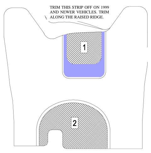
NOTE: IF YOUR VEHICLE HAS A MANUAL TRANSMISSION AND IS A 1997 OR 1998 MODEL REMOVE THE TREAD PLATE FROM AREA "1" SHOWN ABOVE. IF IT IS A 1999 OR 2000 MODEL, TRIM OUT ALL THE MATERIAL INSIDE THE \_ INCH BAND. IF YOUR VEHICLE HAS A CENTER CONSOLE, TRIM THE MATERIAL AWAY FROM AREA "2" SHOWN ABOVE. A UTILITY KNIFE OR HEAVY SCISSORS WORK WELL FOR TRIMMING
