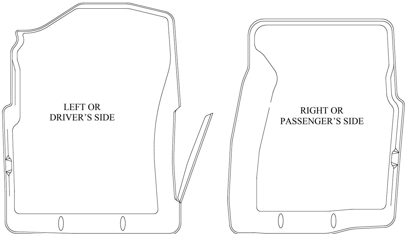
IF YOUR VEHICLE IS EQUIPPED WITH A MANUAL TRANSFER CASE SHIFTER, YOU WILL NEED TO TRIM YOUR LINER AS SHOWN ABOVE. TRIM USING THE MOLDED IN TRIM GROOVE AS A TRIMMING GUIDE. A UTILITY KNIFE OR HEAVY SCISSORS WORKS WELL FOR TRIMMING YOUR LINER.
