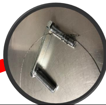
Paired bolt with wire guide
