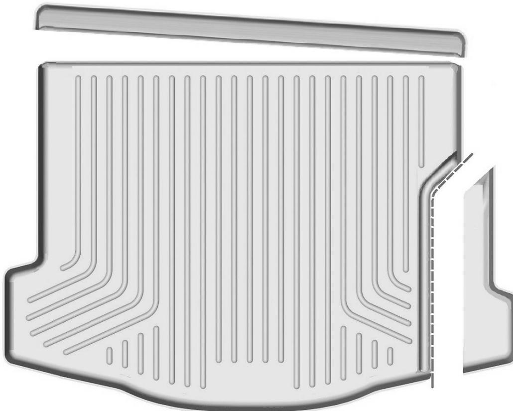
AS BOXED, YOUR LINER WILL NOT FIT FOCUS MODELS WITH A FACTORY SUBWOOFER IN THEIR TRUNK COMPARTMENT. YOUR LINER IS DESIGNED TO ACCOMMODATE THE SUBWOOFER VIA TRIMMING. TO TRIM, LOCATE THE MOLDED IN STEP IN THE LINER THAT ACTS AS A TRIMMING GUIDE (SEE DIAGRAM ABOVE / PHOTOS ON BACK OF PAGE). THEN, USING HEAVY SHEARS OR A UTILITY KNIFE, REMOVE THE AREA OF LINER THAT THE SUBWOOFER WILL OCCUPY.
