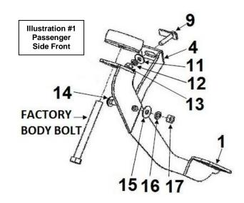
**Step-3** Rremove the passenger side middle body mount bolt. **Photo #2**Keep all existing washers and bushing in place, and attach the front bracket to the vehicle using the factory body mount bolt. Leave the bolt loose for final adjustment. **Illustration #2**
