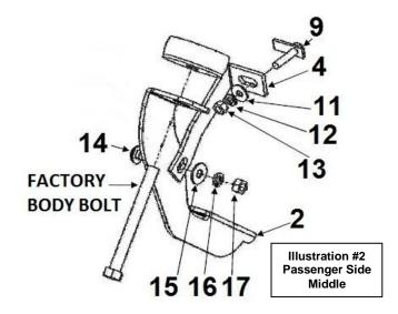
**Step-5** Remove the passenger side rear body mount bolt. **Photo #3** Keep all existing washers and bushing in place, and attach the front bracket to the vehicle using the factory body mount bolt. Leave the bolt loose for final adjustment. **Illustration #3**
