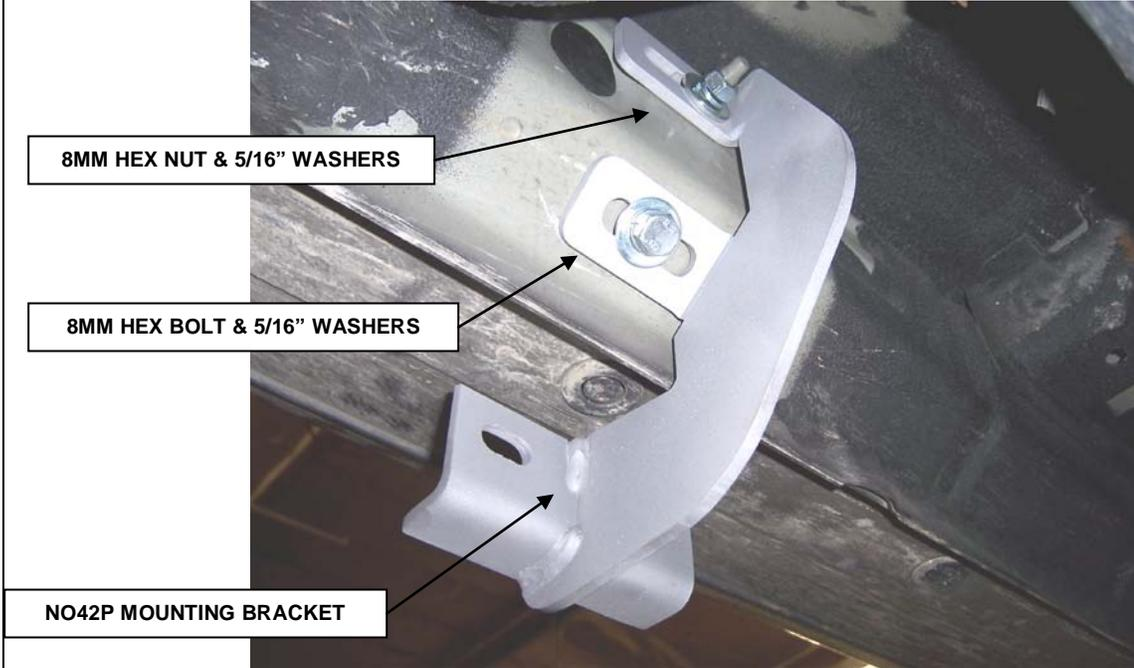
**STEP 3.** Loosely attach one of the NO42P mounting brackets to the body using the 8mm x 25mm hex bolts, 8mm hex nuts, 5/16" flat washers and 5/16" lock washers as shown. Repeat the procedure for the passenger side center and rear brackets.
