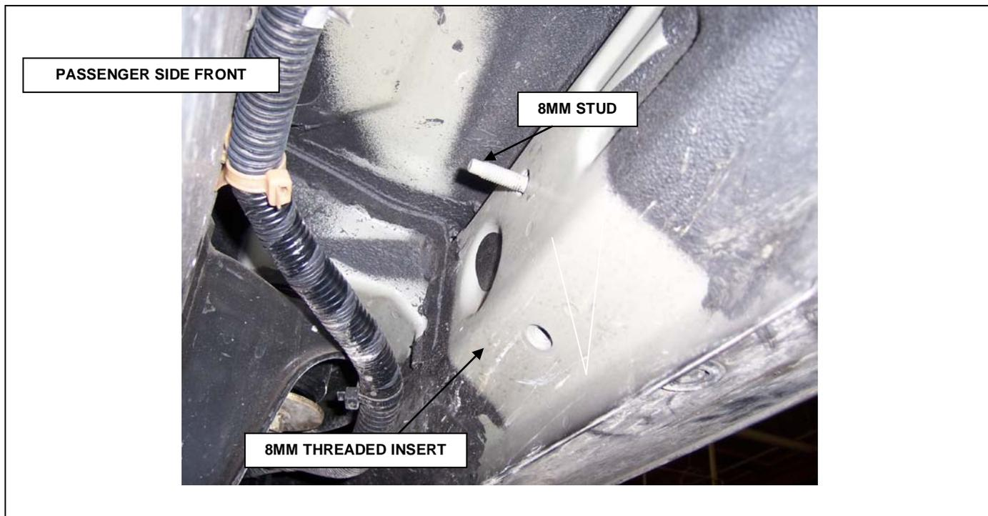
**STEP 2.** This installation uses three mounting brackets per side. Begin by installing the passenger side front mounting bracket. Locate the stud and threaded insert in the under side of the body. Note: you may need to remove the plastic plug to expose the threaded insert.
