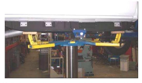
**STEP-5** Position the passenger sidestep up to the mounting brackets and loosely attach it to the brackets using the 3/8" x 1 1/4" hex bolts, flat washers, lock washers and nuts. Align sidestep with the body and then tighten all mounting bracket and sidestep nuts and bolts. Repeat the above installation steps to install the driver side mounting brackets and side step.
