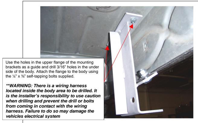
**STEP-4** Loosely attach the lower flange of the mounting brackets to the bottom of the body pinch mold using the 3/8" x 1" carriage bolts, flat washers, lock washers and nuts as shown.
