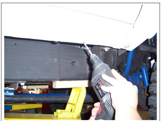
**STEP-3** Confirm the measurements, center punch and drill 3/8" holes through the body pinch mold. Repeat the above procedure for the driver side.
