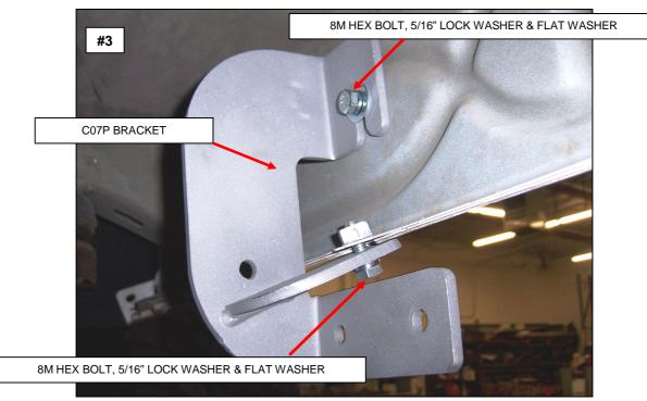
**Step-2** Attach one of the C07P brackets to the rocker panel and pinch mold using (2) 8M hex bolts, (2) 5/16" lock washers and (2) 5/16" flat washers. Leave the bolts loose for final adjustment. **Photo #3**
