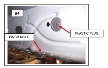
**Step-4** Measure from the front fender bolt reward approximately 75 1/8" for the rear bracket and locate the hole in the body pinch mold and the plastic plug in the rocker panel. Remove the plastic plug from the rocker panel and install (1) 5/16" U-Nut in the rocker panel.
