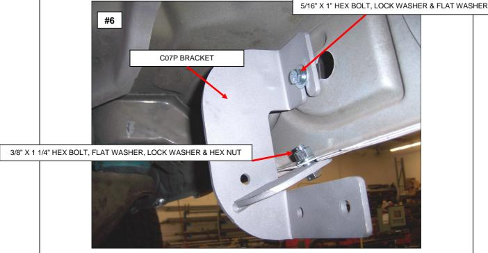
**Step-5** Attach each bracket to the rocker panel using (1) 5/16" x 1" hex bolt, (1) 5/16" lock washer, (1) 5/16" flat washer and to the pinch mold using (1) 3/8" x 1 1/4" hex bolt, (1) 3/8" lock washer, (1) 3/8" flat washer and (1) 3/8" hex nut. Leave the nut and bolts loose for final adjustment. **Photo #6 & #7**
