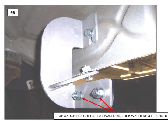
**Step-7** Align the side step with the vehicle and tighten all bracket and side step nuts and bolts. Repeat the above steps to install the driver side brackets and side step.
