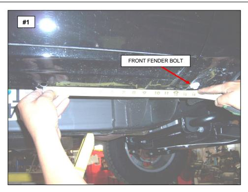
**Step-1** This installation uses three brackets per side. Begin by installing the passenger side front bracket. Measure from the front fender bolt rearward approximately 14" and locate the 8M nut welded to the body pinch mold and the 8M threaded insert in the rocker panel. **Photo #1 & #2**
