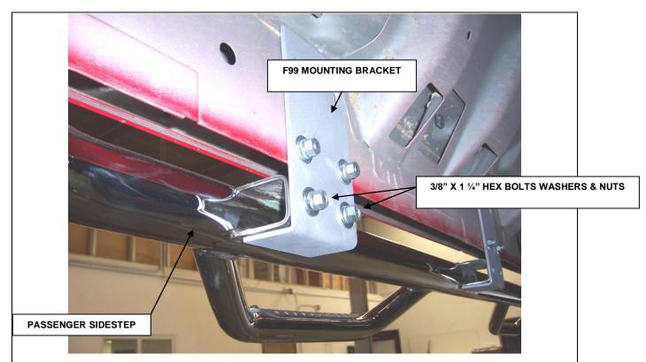
**Step-7** Position the passenger sidestep up to the mounting brackets and loosely attach it to the brackets using the 3/8" x 1 1/4" hex bolts, washers and nuts as shown.
