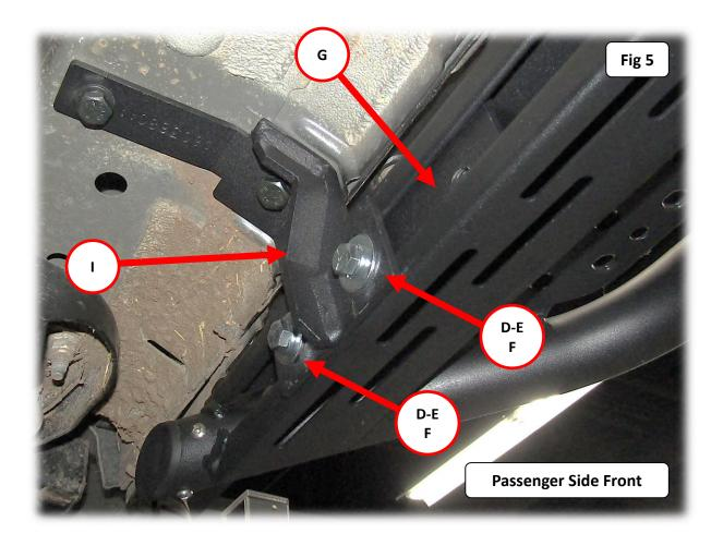
**Step-6** Align the Dominator DSS side step with the vehicle and tighten all bracket and side step nuts and bolts,. Repeat the above steps to install the driver side brackets and Dominator DSS side step.
