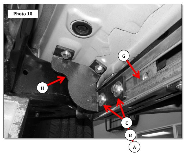
**Step-9** Align the Dominator DSS side step with the vehicle and tighten all bracket and side step nuts and bolts,. Repeat the above steps to install the brackets and Dominator DSS side step on the driver side of the vehicle.
